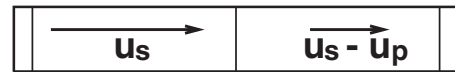
FIG. 1. Schematic stationary shockwave. Cold fluid enters at the left cold boundary, with speed u_s ; hot fluid leaves at the right hot boundary, with speed u_s - u_p . We choose a coordinate frame which moves leftward, at speed u_s relative to the laboratory frame. The shockwave remains stationary in this coordinate frame.
